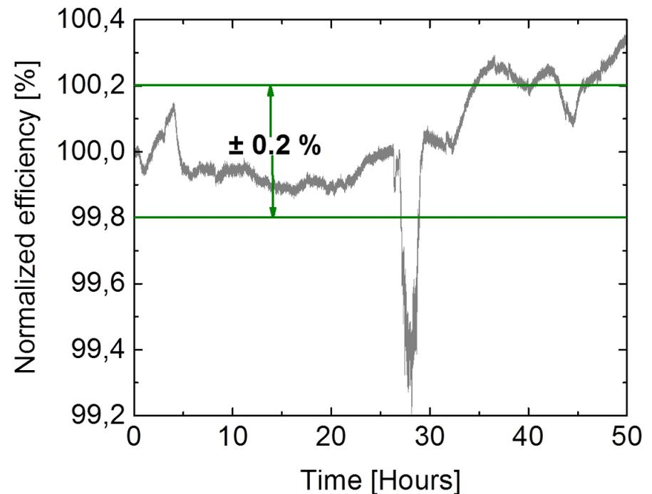
■ long-time stabilization with MPP load resistor at 1/10 sun intensity
