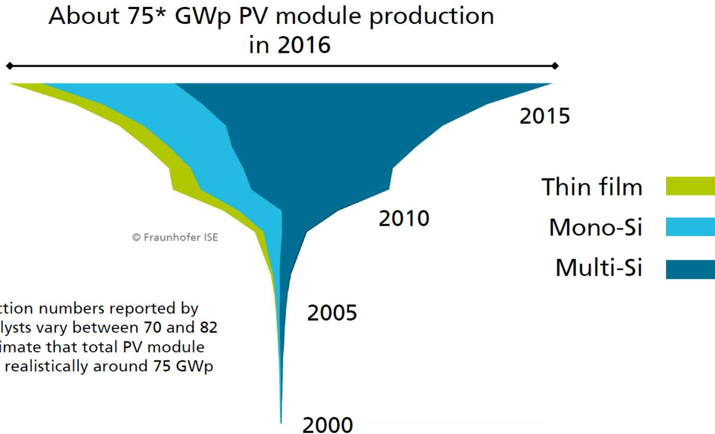
\*2016 production numbers reported by different analysts vary between 70 and 82 GW<sub>p</sub>. We estimate that total PV module production is realistically around 75 GW<sub>p</sub> for 2016.
