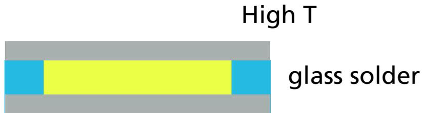
1. Encapsulating „inorganic part“ by thermal glass fusing
